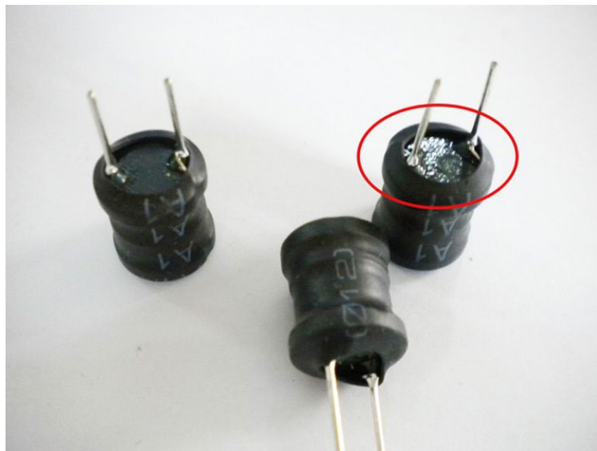
Figure 3: Common soldering defects — spatter, spikes, and inconsistent joints
